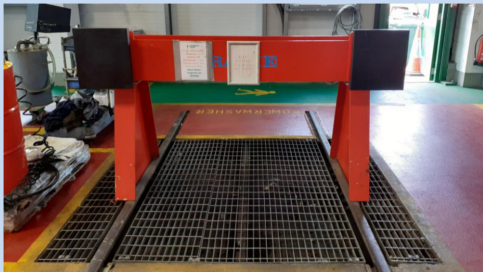
Photograph 3 – Example of fixed buffer stop insitu:
