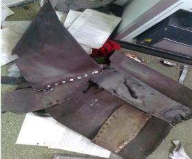
Figure 2 - Damage to driving cab ceiling
