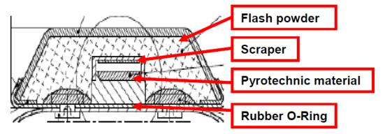
Figure 9 - Design of the Alsetex fog signal
