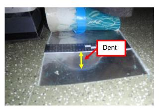
Figure 22 - Dent in the floor
