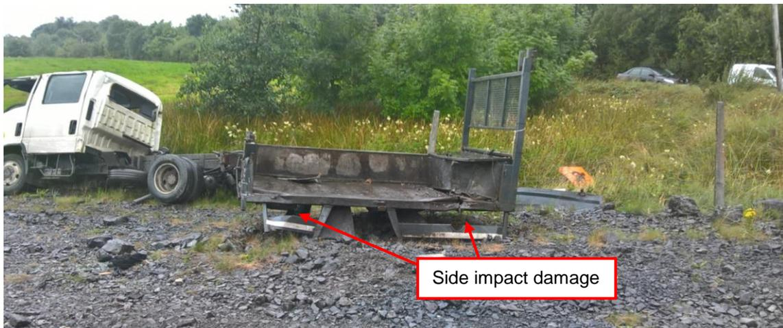
**Figure 5 – Damage to the Truck and fencing**
