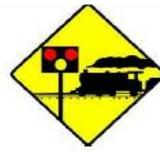
W 120: Level Crossing with Flashing Red Signals
