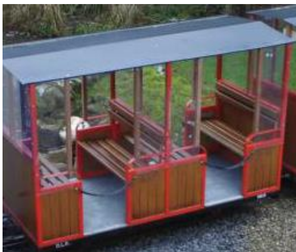
Figure 3 – Open carriage with chains
