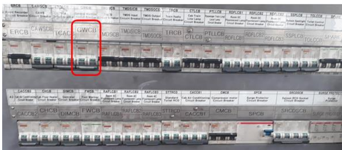
Figure 9 – Tripped GWCB on the cab circuit breaker panel
