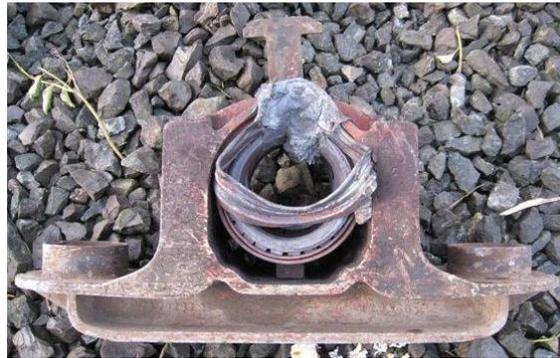
Photo 2 – Failed Bearing & Axlebox
