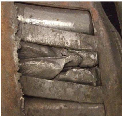
Photo 4 – Fractured Roller
