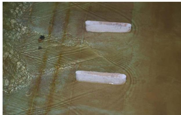
Photograph 8 – 3-D model of movement of hydraulic jump
