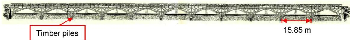
Figure 2 – Original timber structure with timber piles
