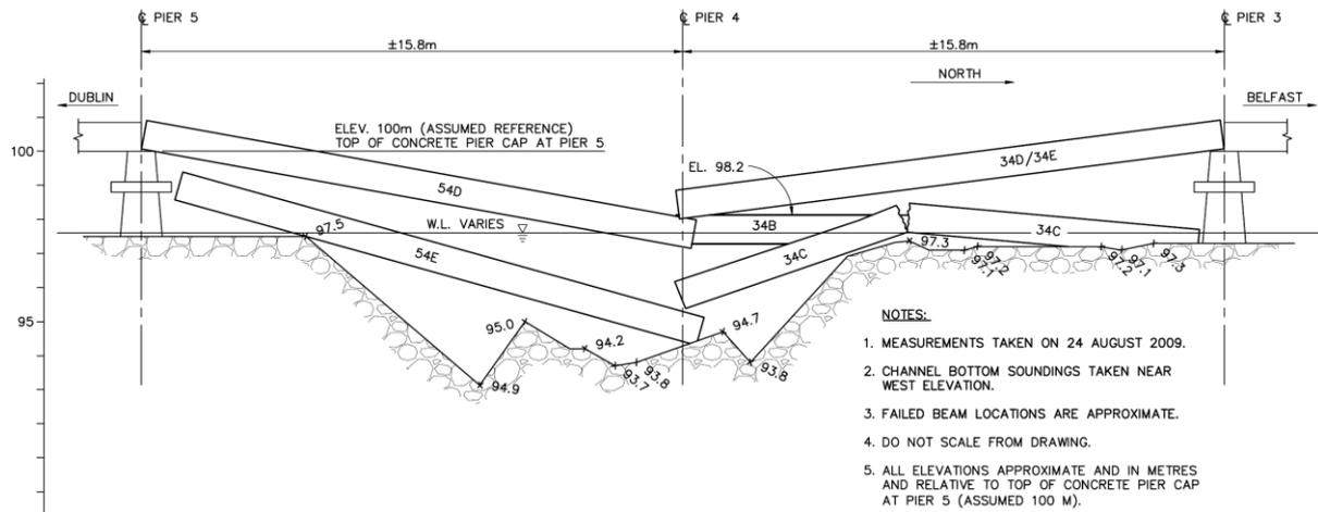
Figure 23 – Post accident survey illustrating asymmetrical scour hole
