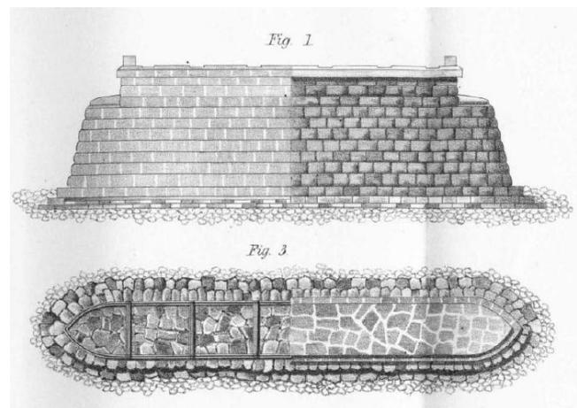
Figure 5 – Elevation and plan of the masonry piers
