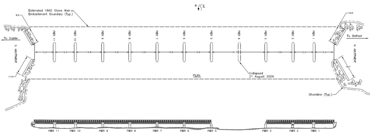
Figure 6 – Plan and elevation illustrating pier numbering
