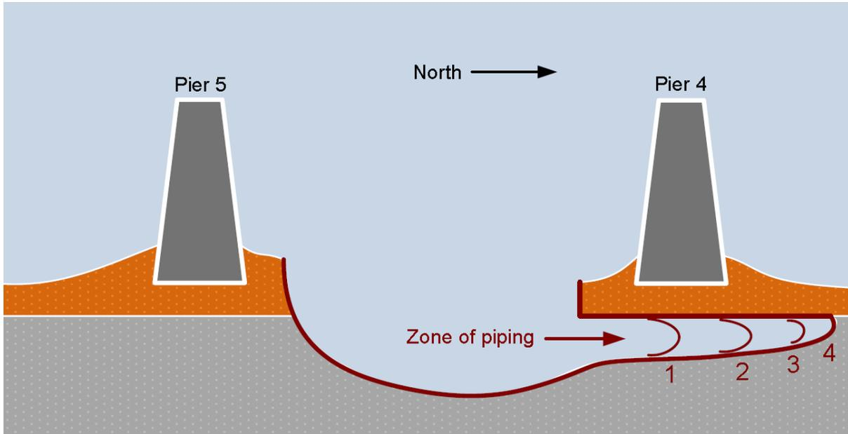
Figure 20 – Piping under Pier 4.
