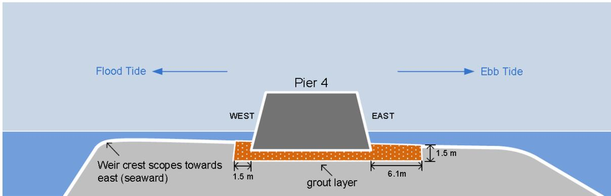
Figure 13 – Grout layer (grouted rock armour) inserted in 1967 – 1968
