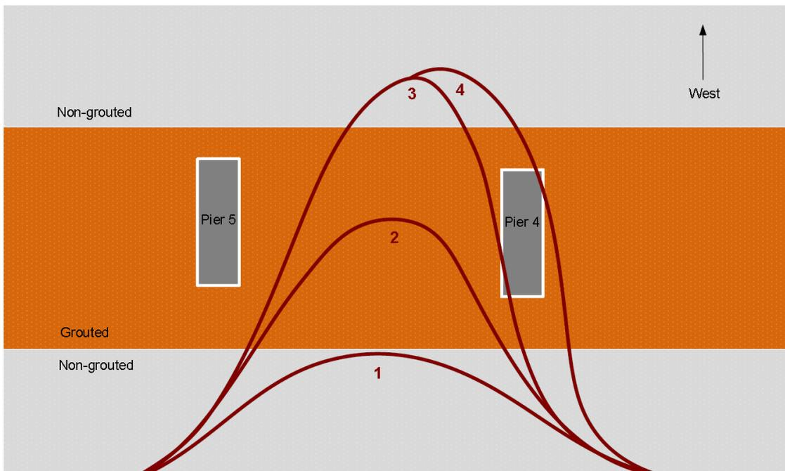
Figure 21 – Undermining of Pier 4 as a result of piping
