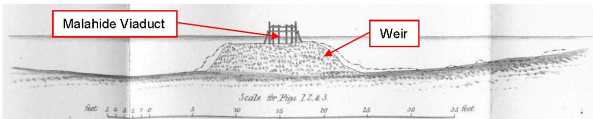
Figure 3 – Malahide Viaduct on weir construction
