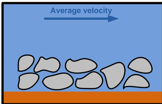
Figure 10 – Stable cobbles during average velocities
