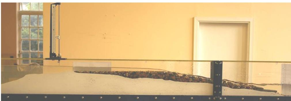
Photograph 6 – 2-D model in laboratory flume
