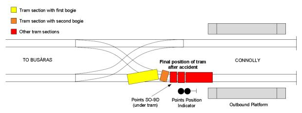
Figure 2 – Final position of the tram after accident
