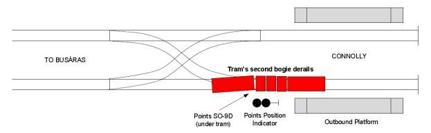
Figure 7 – Second bogie travelling in wrong direction.
