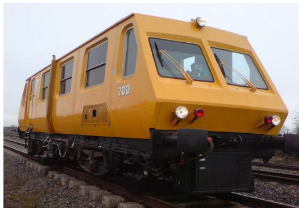
Photograph 7 – Track Recording Vehicle
