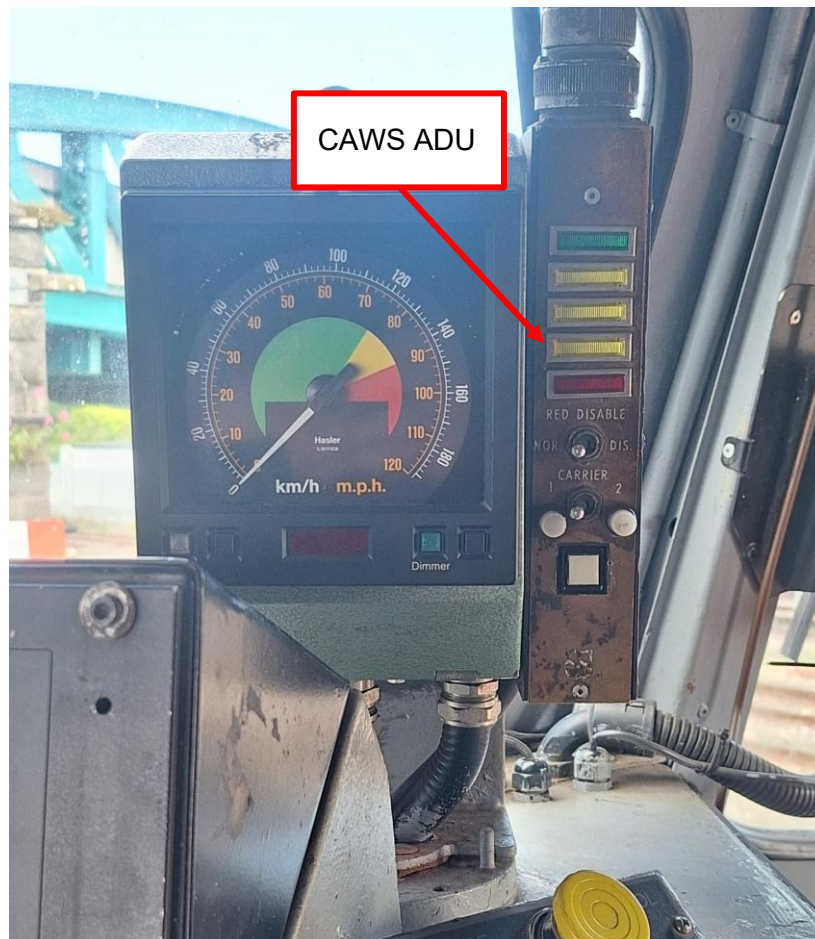
Figure 3 – CAWS ADU in a Class 071 locomotive
