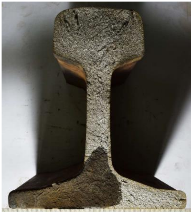
Figure 9 – Complete fracture face showing rail foot crack
