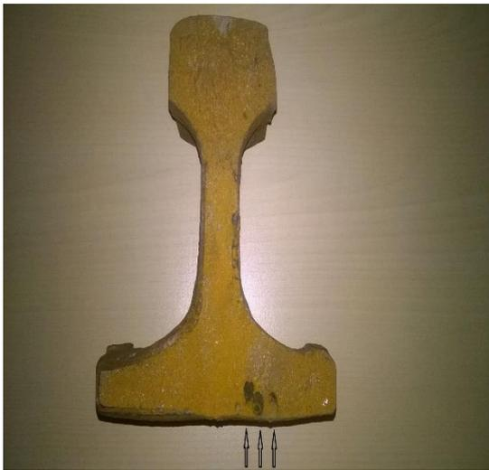
Figure 13 – Rail foot defects
