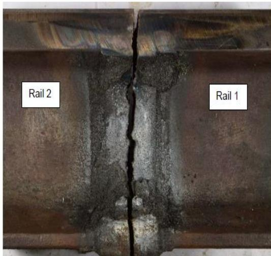
Figure 9 – Transverse failure through the centreline of the weld
