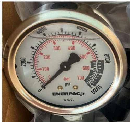
Figure 6 – Pressure gauge
