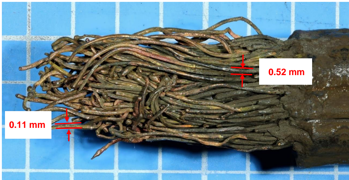
Figure 12 – Failed Current Return cables strands
