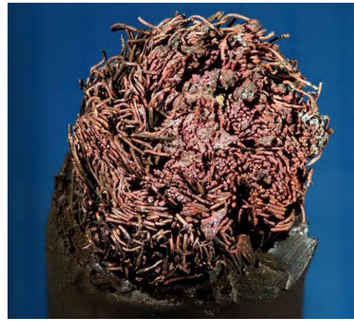
Figure 14 – Central fused cable strands
