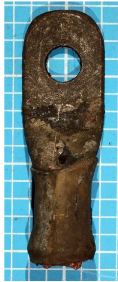
Figure 16 – S3 Earth Shunt Cable Lug closest to the failure
