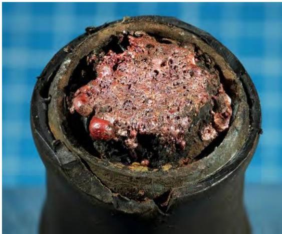
Figure 13 – Lug side fused cable strands
