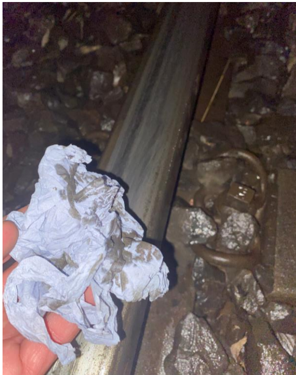
Figure 12 – Contaminated railhead on the Up Road
