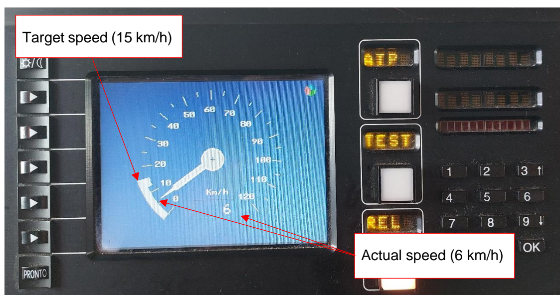
Figure 10 – Driver's in-cab display of the ATP
