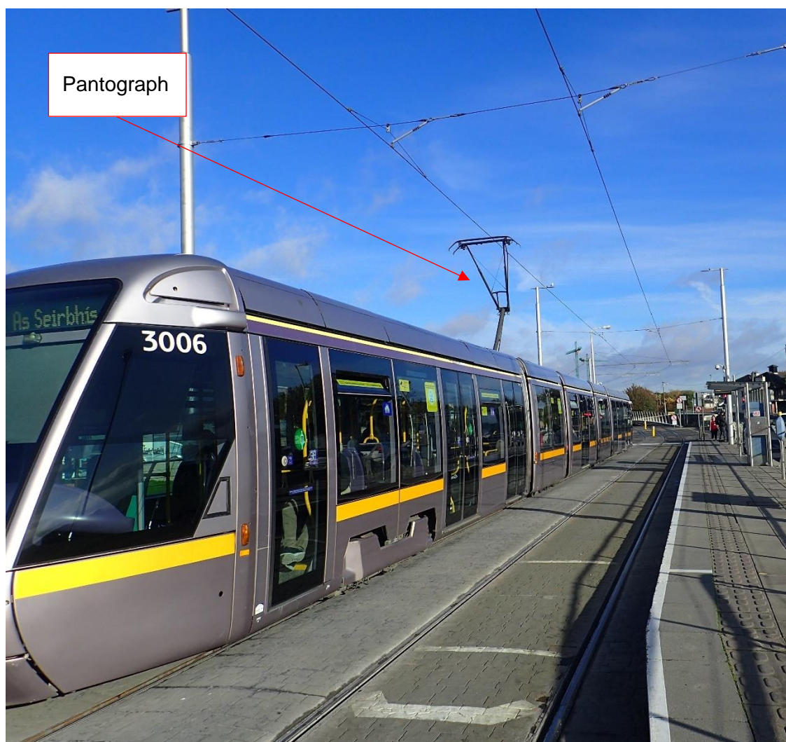
Figure 3 – Tram pantograph interface with OCS
