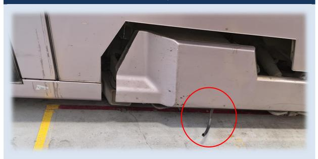
At approximately 08:08 hrs on the 25<sup>th</sup> October 2022, a tram driver leaving Connolly Stop observed what he thought was a hose sticking out from a side skirt on Tram 3012 and reported the incident to LNMC.
