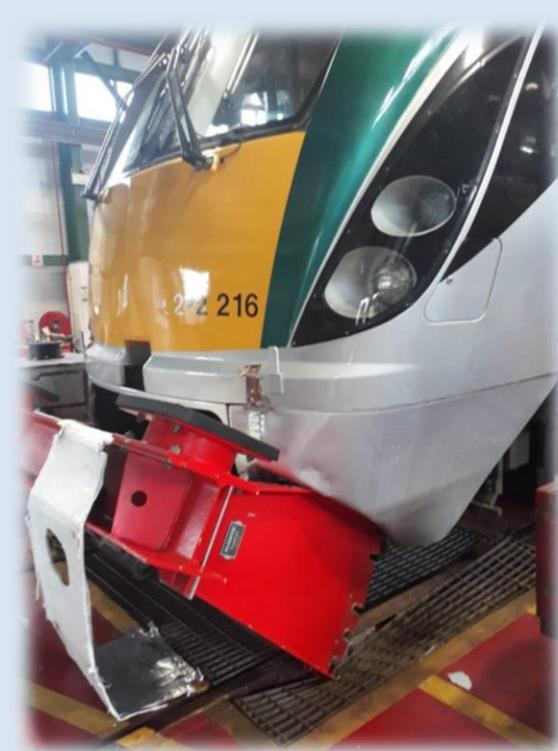
While undergoing maintenance intervention on Pit Road 8, LTCD, ICR 16 was moved approximately 8.25 meters under its own power before colliding with a fixed buffer stop.
