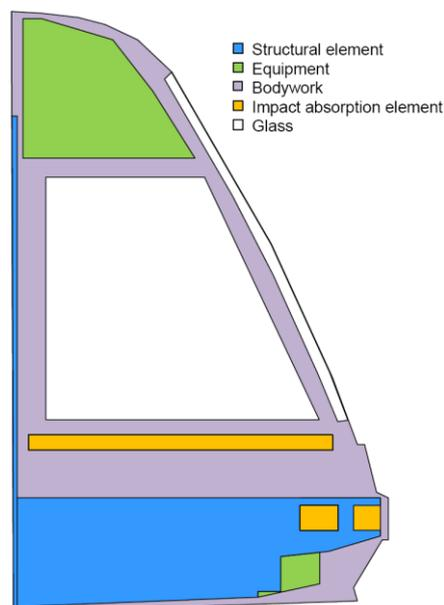
Figure 6 – Front end cab design
