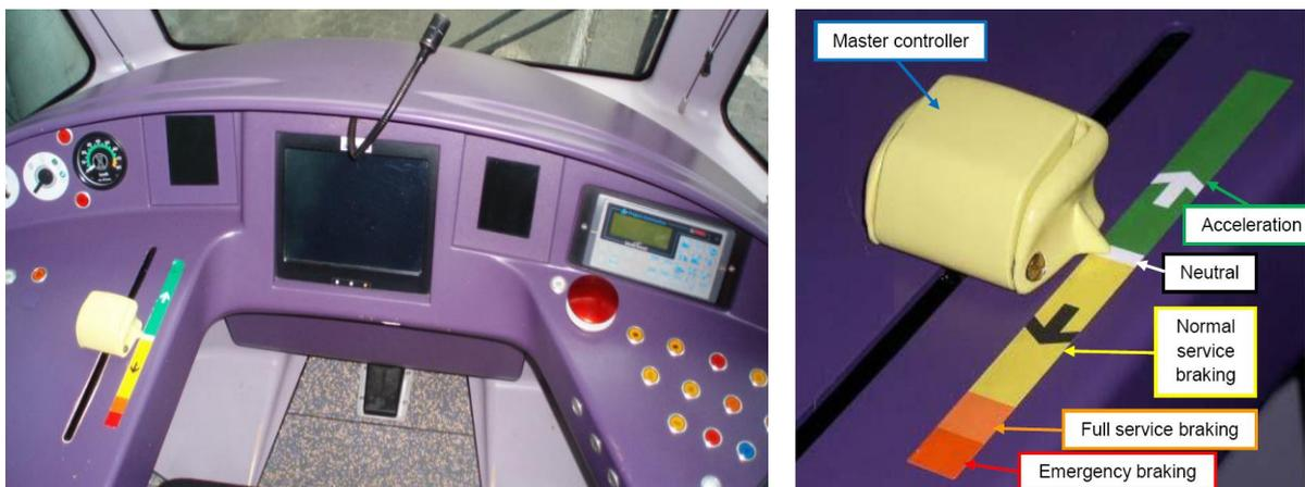
Figure 7 – Driving console with close up of master controller
