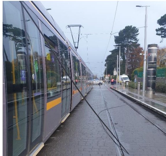
Figure 16 – OCS hanging over Tram 5010 Figure 17 – OCS wire on outbound track
