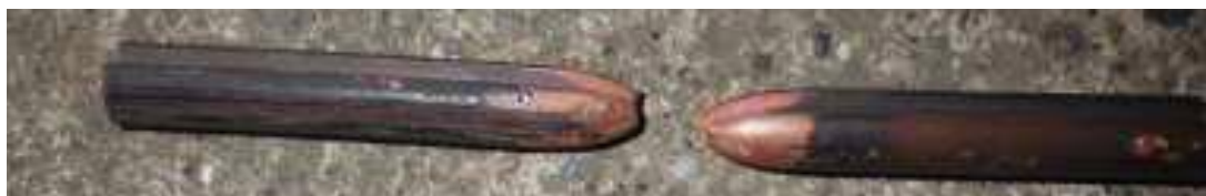
Figure 22 – Failed OCS wire from Milltown
