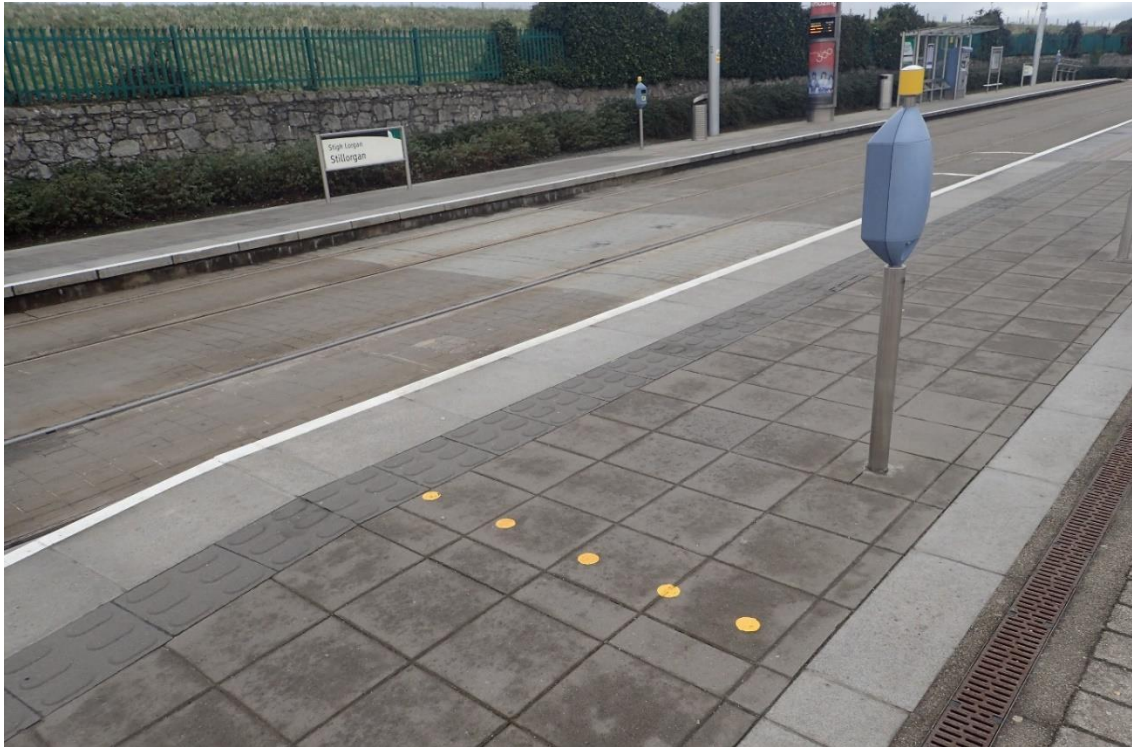
Figure 2 – Yellow dots indicating the stopping position for trams at Stillorgan
