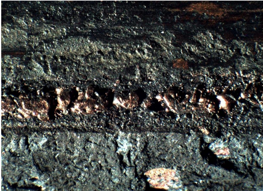
Figure 10 – Close-up of black coating on the OCS wire
