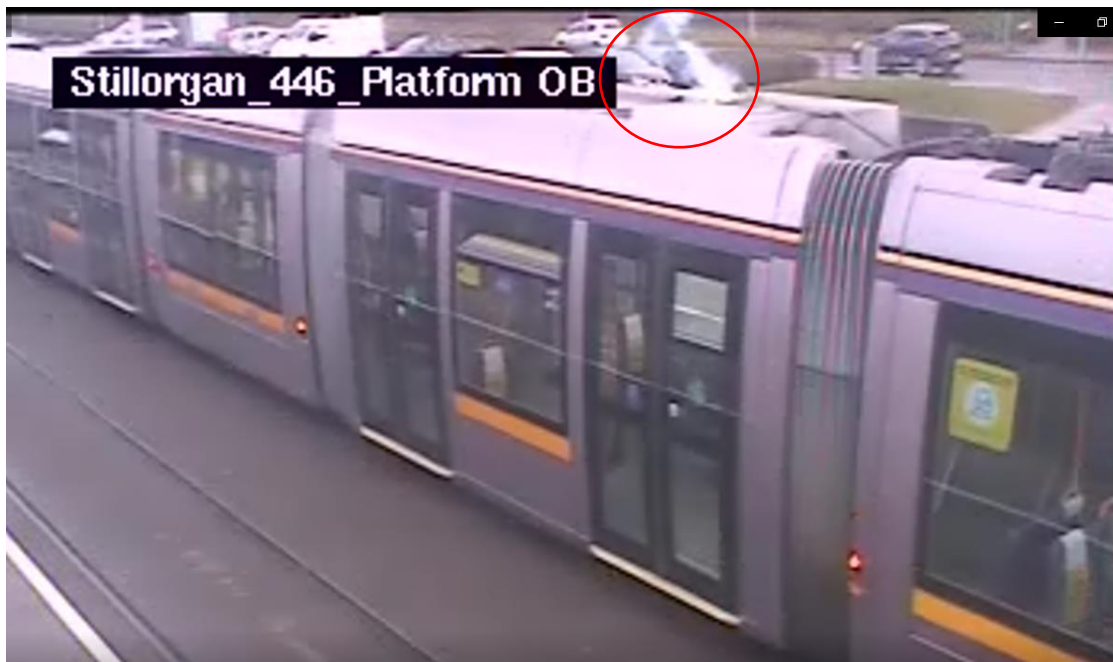
Figure 14 – Short-circuit between the OCS and roof of Tram 5010
