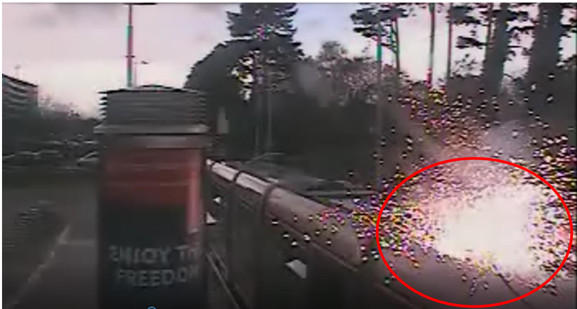
Figure 20 – Second short-circuit between the OCS and roof of Tram 5010
