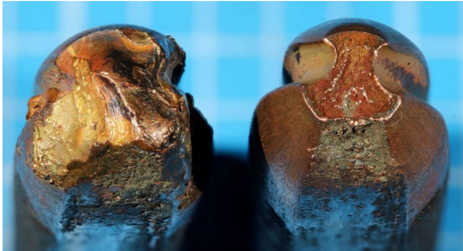
Figure 9 – Images of failed OCS wire from Stillorgan
