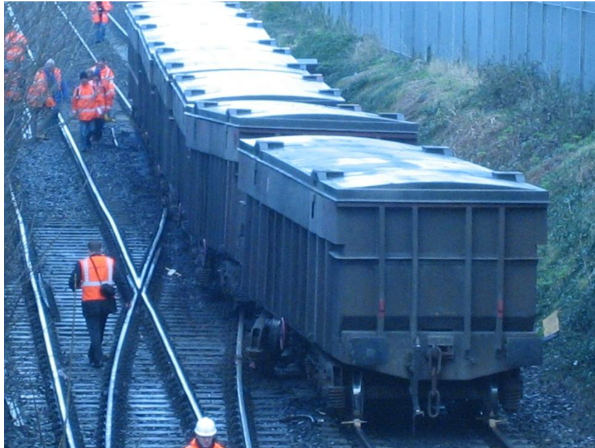
Photograph 2: Derailed Tara Mines freight train
