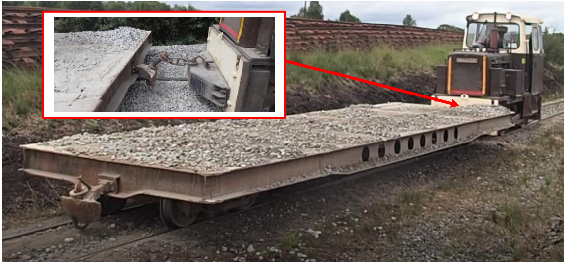
Figure 2 – Locomotive coupled to Flat Wagon (coupling arrangement inset)
