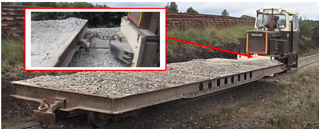
Figure 8 – Locomotive coupled to Flat Wagon (coupling arrangement inset)
