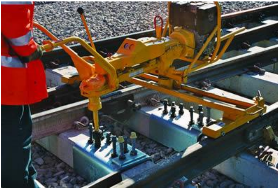
Figure 7 – Geismar Universal Power Spanner mounted on rails
