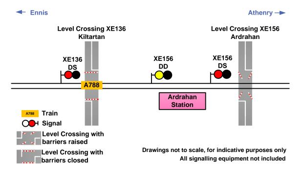
Figure 11 – At 19:48 hrs Train A788 triggers the auto-initiation for the lowering of barriers of Level Crossing XE156
