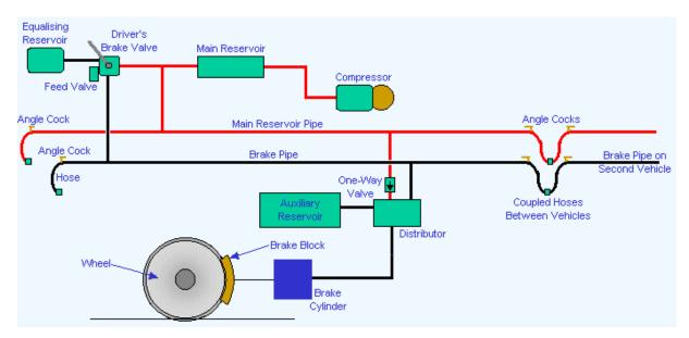
Figure 27 – Block diagram of two-pipe air brake system
