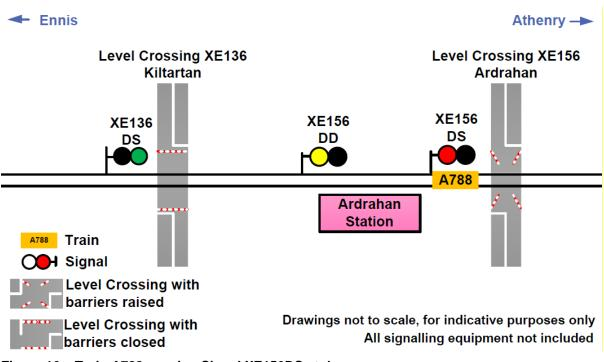
Figure 16 – Train A788 passing Signal XE156DS at danger
