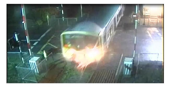
Figure 17 – Train A788 passing through Level Crossing XE156 Ardrahan with the barriers raised to road traffic.
