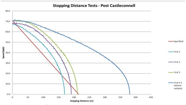
Figure 28 – Results of IÉ dynamic brake testing
