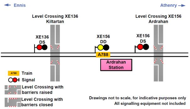
Figure 13 – Train A788 passed Signal XE156DD indicating that the next signal, Signal XE156DS is at danger
