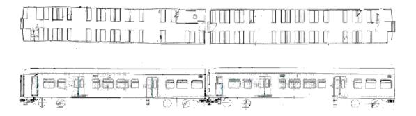
Figure 8 – Unit configuration of Class 2600
