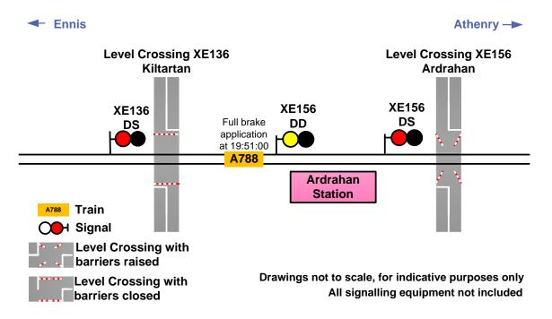
Figure 12 – Initial brake application at 19:50:56 & full brake application at 19:51:00
