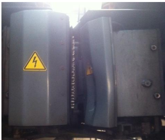
Figure 4 Damaged to autocoupler
