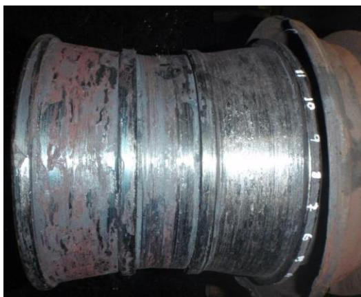
Figure 6 - Bearing cone raceways
