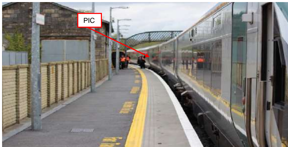
Figure 61 – Curved platform & driver's view of PIC
