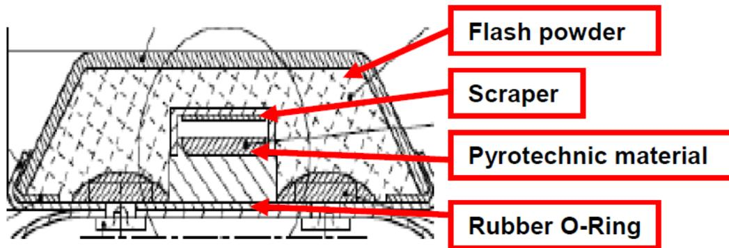
Figure 9 – Design of the Alsetex fog signal
