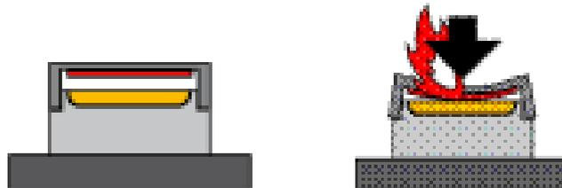
Figure 10 – Activation process for Alsetex fog signal
