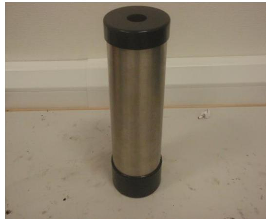
**Figure 15 – Stainless steel tube with cap**
