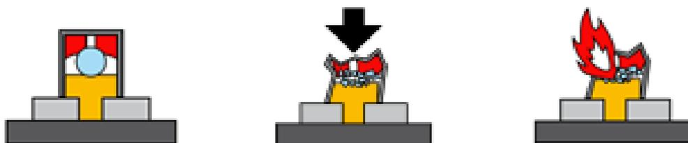
**Figure 8 – Activation process for Lacroix fog signal**
