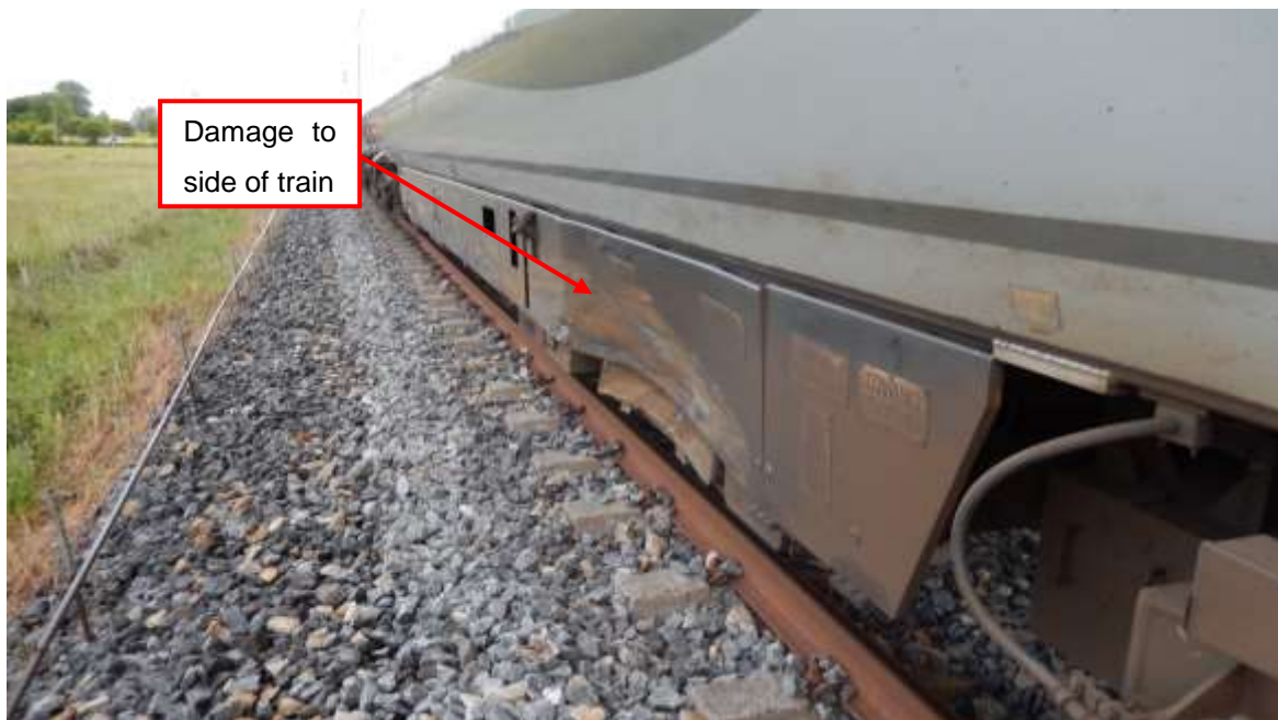
Figure 7 – Damage to the side of the train
