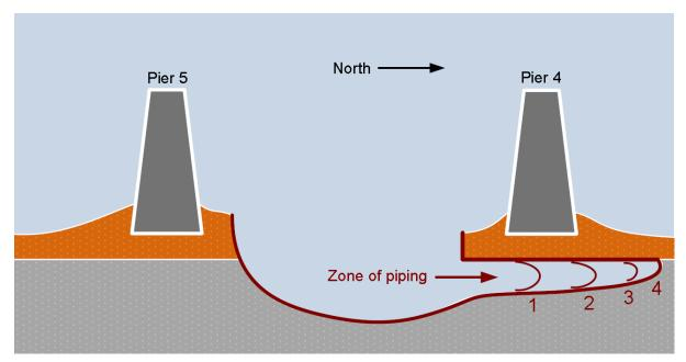
Figure 20 – Piping under Pier 4.
