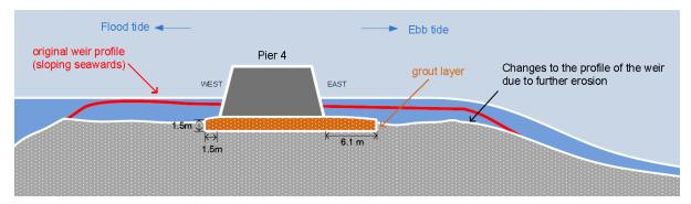
Figure 16 - Erosion of the eastern side of the weir
