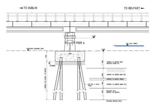
Figure 28 - Piles in Pier 4
