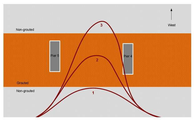
Figure 19 – Westward propagation of the hydraulic jump and erosion due to scour action
