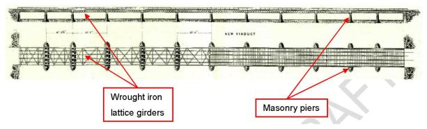
Figure 4 – New masonry and wrought iron Malahide Viaduct constructed in 1860
