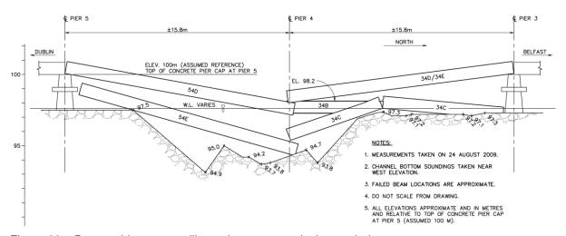
Figure 23 - Post accident survey illustrating asymmetrical scour hole
