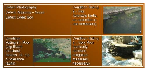
Figure 27 – Defect photography and condition ratings for scour
