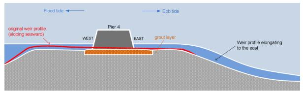
Figure 15 – Weir profile remains elongated to the east, with the grout layer (rock armour) stabilising the scouring
