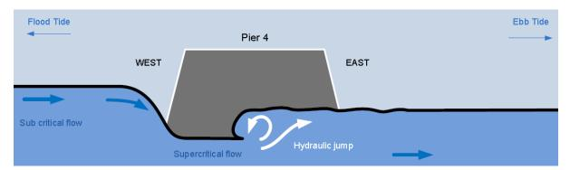
Figure 18 – New position of hydraulic jump, between piers 4 and 5
