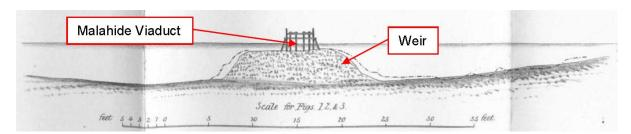
Figure 3 – Malahide Viaduct on weir construction
