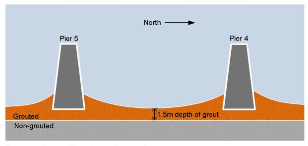
Figure 14 – Elevation illustrating the dipped profile between the piers
