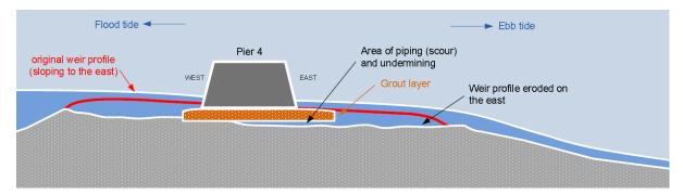
Figure 22 – Transport of materials after the movement of the hydraulic jump
