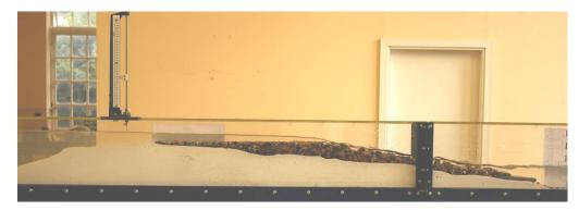
Photograph 6 – 2-D model in laboratory flume
