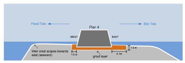
Figure 13 - Grout layer (grouted rock armour) inserted in 1967 - 1968
