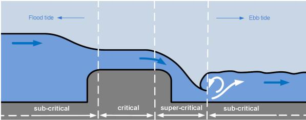
Figure 9 - Water flow over a weir
