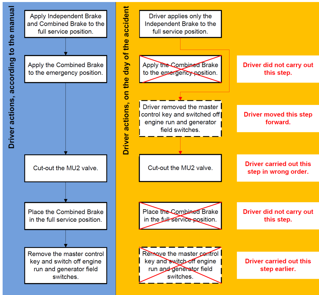
Figure 10 – Actions to be taken by train drivers in relation to vacating a cab according to the manual compared with actual actions taken by Train Driver on the day of the accident.
