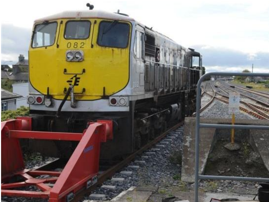
Figure 3 – Locomotive at stopping position at buffer stop
